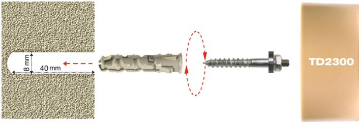
When the surface allows for the drilling of a deeper hole, such as cement or concrete, a plastic dowel can be used.
