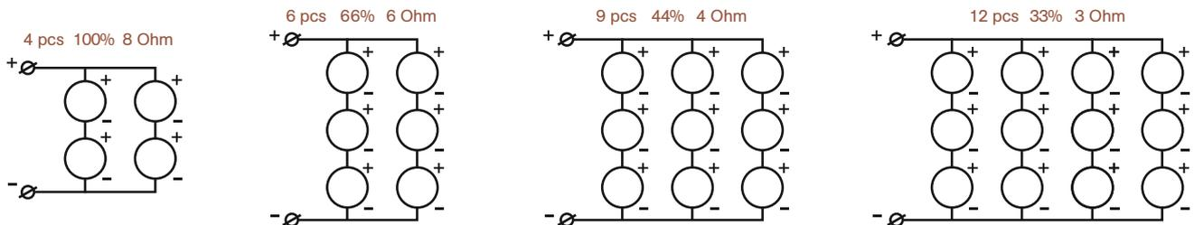
The output power is divided between the transducers, so when there are more transducers, each separate unit will receive less power.
