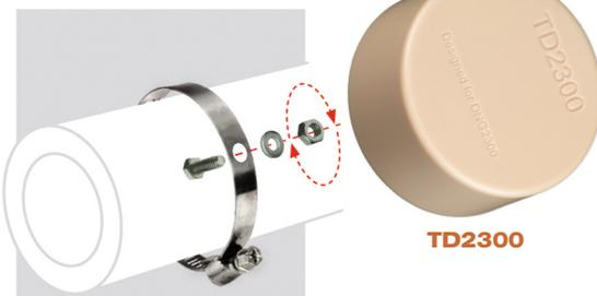
Since water is a good conductor of sound, it is recommended to install the TD2300 transducer onto each pipe going in, or out, of the protected room. You will need some extra accessories which are not included in the supplied set: i.e. interlocked hose clamp 100-150 mm, bolt M4x8, washer and nut.
