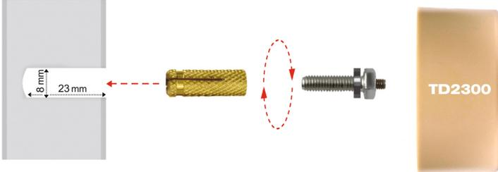
For walls with fragile surfaces such as drywall, plaster, or thin paneling, the transducer can be attached with the help of the supplied bolt and wall anchor.
