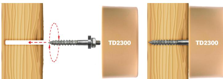
A double ended screw is provided in the supplied set. One end has machine screw threads for the transducer; the other has coarse, tapered threads to be used in such uniform materials such as wood, ply wood, studs, or wood beams.
